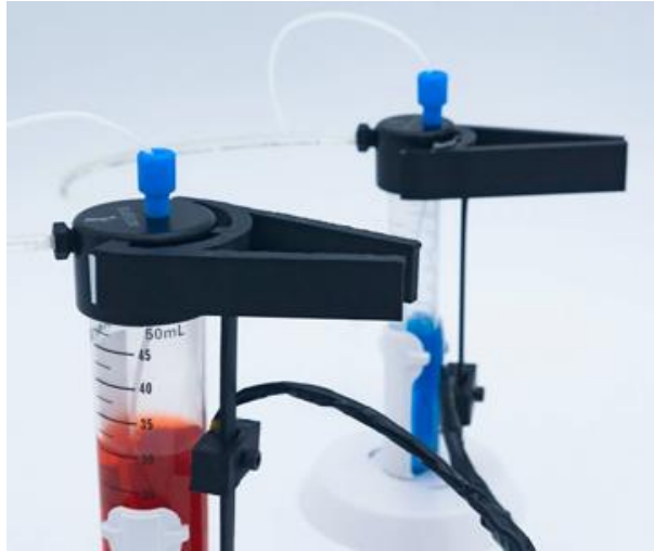
Fig. 3. Reservoir level sensors for fail-safe recirculation of liquid in each circuit. Level sensors are adaptable to a range of tube sizes, from Eppendorf tubes to 15 mL and 50 mL Falcon tubes. User-friendly and intuitive software enables the user to get started in a few clicks and further automate the most complex and long-lasting experiments.
