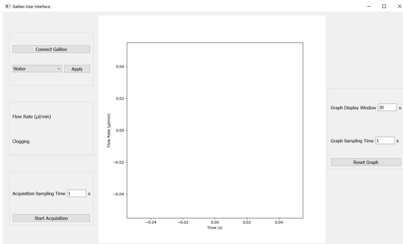
Ensure the Galileo is connected via the provided USB cable to your PC, and the cartridge is properly connected to the base. Once the physical connections are made, you may click the “Connect Galileo” button on the interface, shown below.
